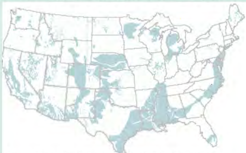
Areas where subsidence has been attributed to groundwater pumping (Land Subsidence in the United States, USGS Circular 1182)
